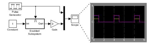
Simulink computes the outputs of the Constant block and Gain Block only when the Enabled Subsystem executes (i.e., at time steps 0, 4, 8, and so on). This is because the output of the Constant block is required and the input of the Gain block changes only when the Enabled Subsystem executes. When CE behavior is off, Simulink computes the outputs of the Constant and Gain blocks at every time step, regardless of whether the outputs are needed or change.
