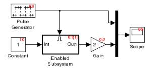
In this example, the sorted order index of the enabled subsystem is  $0:1\{1\}$ . The 0 indicates that the enable subsystem resides in the model's root system.
