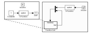
Such models cannot be correctly simulated. Accordingly, Simulink now displays an error message when you attempt to run or update a diagram containing function-call cycles.
